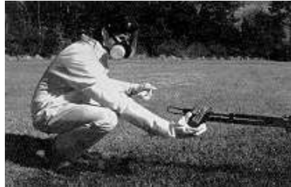
FIGURE 3. DETERMINE THE OUTPUT OF A SINGLE NOZZLE.
