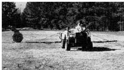
FIGURE 2. DETERMINE MILES PER HOUR BY DRIVING THE SPRAYER THROUGH A 200-FOOT COURSE.
